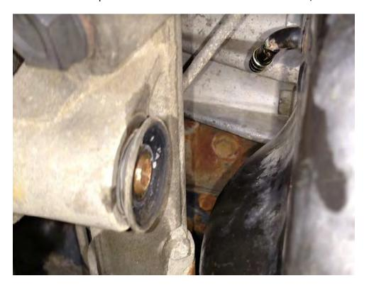
This picture shows how much the ring gear protrudes from the front differential housing.
