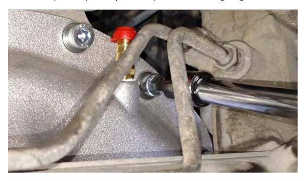
The diff cover did clear the rack bolt, but I elected to cut 1/4 inch off the rack bolt to allow maximum clearance and still leave enough thread to fully tighten the nut.
