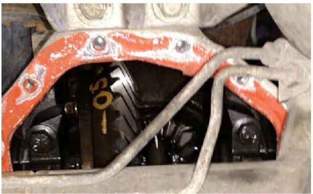
I did a dry fit and all of the bolts lined up. However, I was unable to tighten this bolt (and the one on the opposite side top, same position) with my 3/8 drive hex head driver because of the limited distance between the rack and the bolt head. A modified Allen wrench could be used to tighten this bolt.
