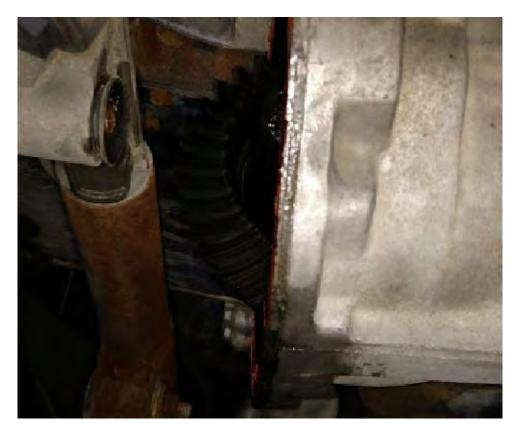
The housing/diff mating surface was thoroughly cleaned and allowed to dry (before pictures).
