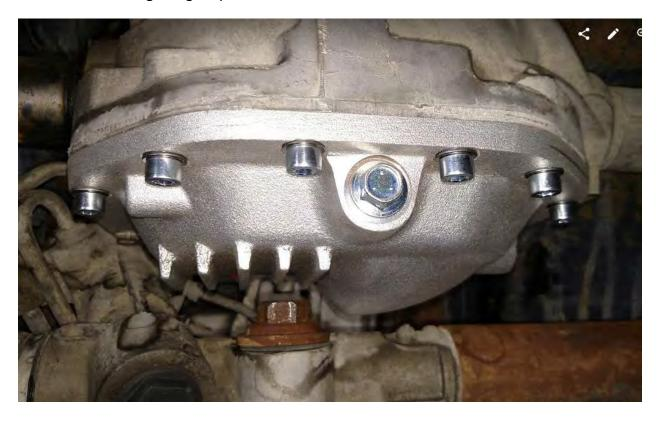
After the dry fit, I applied 1/8 inch of black silicone to the housing in a pattern specified in the instructions provided by PML.
