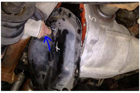
Once the bolt was pushed back and the vent tube hose removed, I was able to remove the stock cover.
