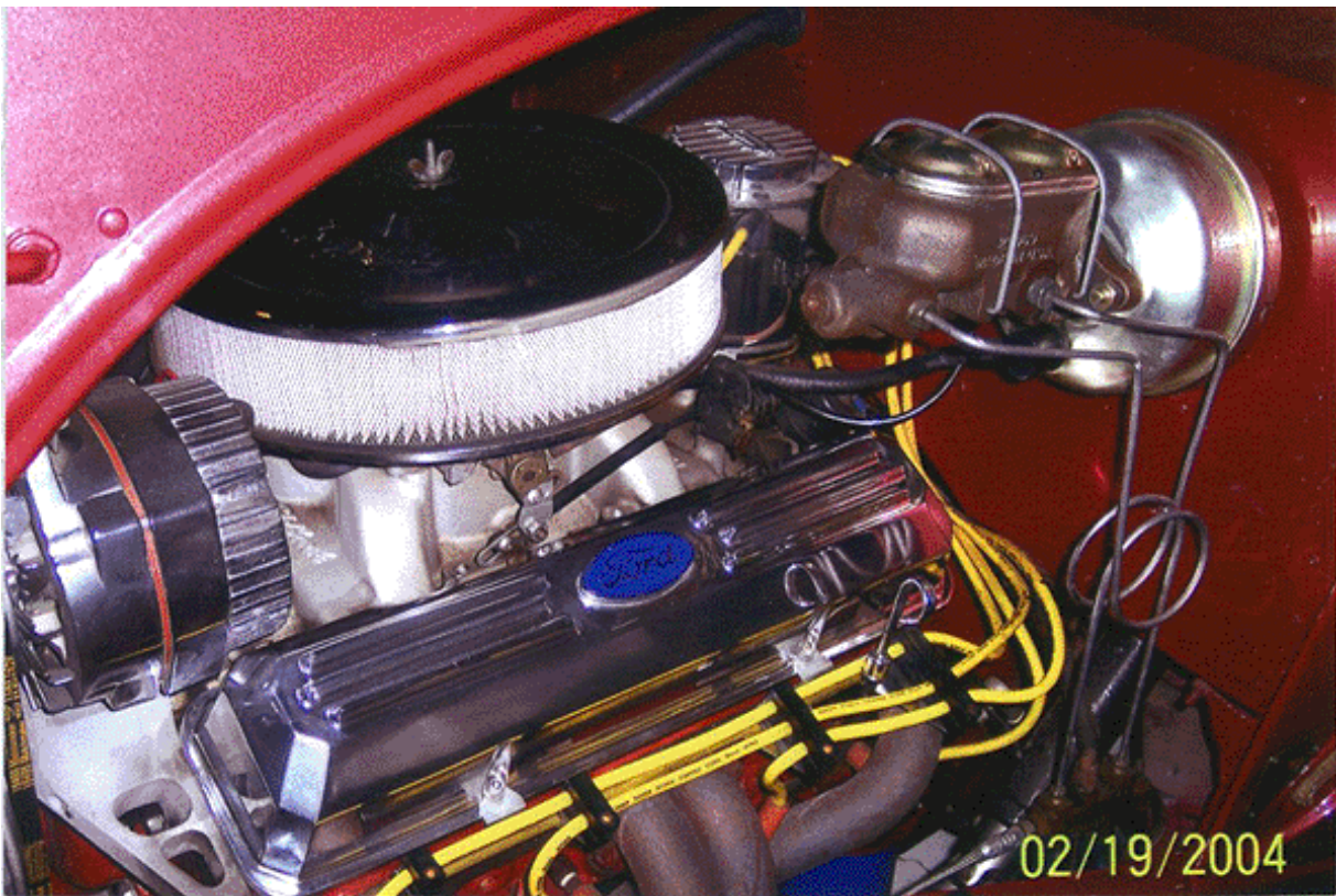
PML part number 8357-6, polish finish, installed.
