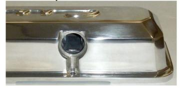
PML machines the holes for a clean appearance and a good fit to the grommet or breather. To achieve this, PML sets up on each cover and uses four different tools.
