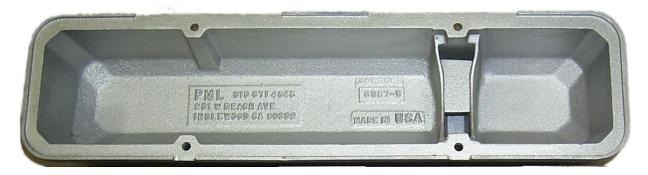
When the PML supplied breather is installed, it sits inside the baffle.
