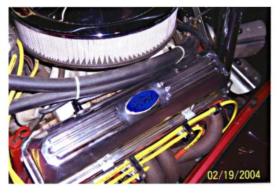
This example is from a 1934 Ford Cabriolet with a small block Chevy engine. The PCV is on the passenger's side (near the firewall).
