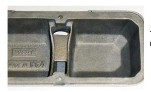
This shows the inside of the cover after we have machined it for a PCV/breather hole.
