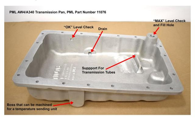
Once installed, the bottom of the transmission pan should be parallel to the ground for the fluid level check system on the PML pan to be accurate.
