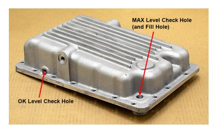
Check the fluid level as you would with the stock pan (temperature, parked on a level surface).
