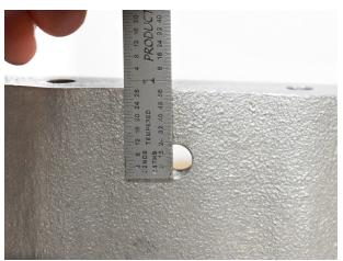
In addition to these rough manual measurements, PML laser scanned the parts and used computeraided design software to determine the locations. There is some variability since there is a big range between OK and MAX levels and the transmission housing flange is not parallel to the ground.
