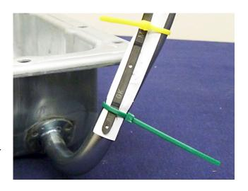
So with a PML AW4/A340 pan you do NOT use a dipstick. The OK and MAX fluid level checks are holes on the pan. Plugs for the holes are included.
