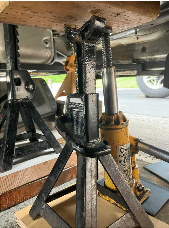
Bottle jack under transmission support block. Jackstand in place under rear transmission mount.
