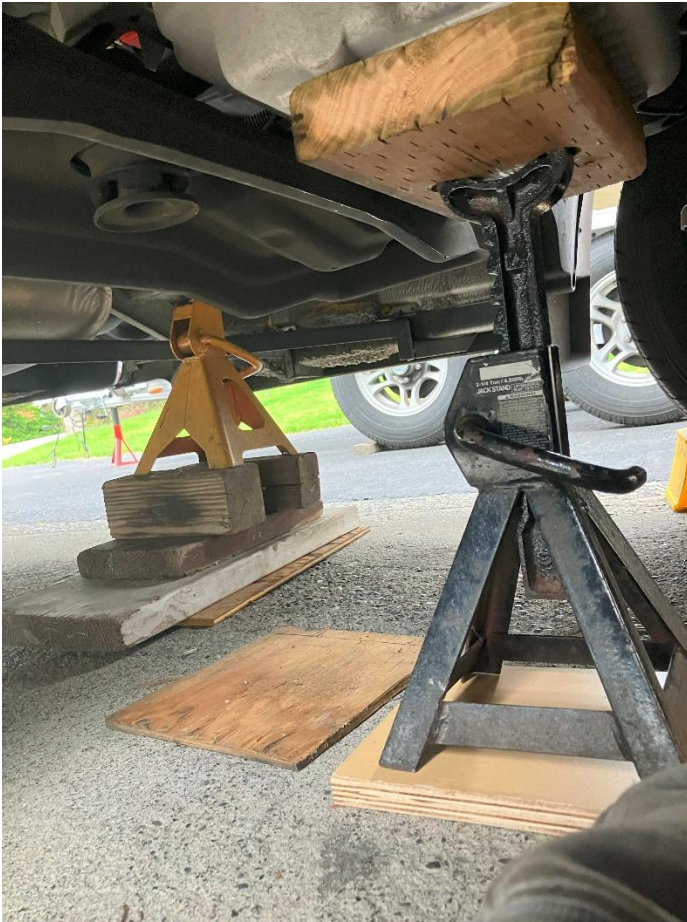
Jackstand w/wood block under transmission pan.
