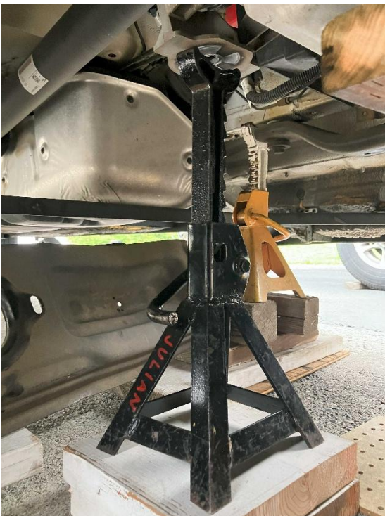
Jackstand in place under rear mount ready for load transfer.
