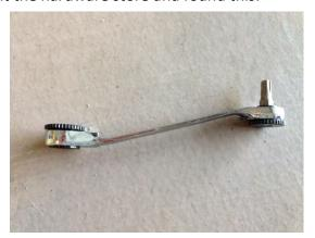
Which allowed me to use a T30 bit in this wrench. That worked for me to get out the rear-most 2 Torx bolts.
