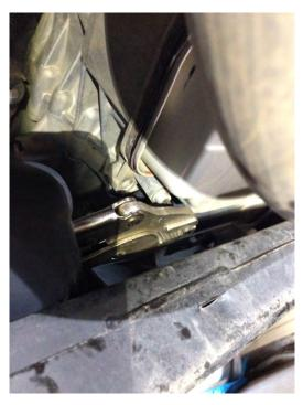
The rear-most 2 Torx-head bolts that hold on the stock pan were above the main cross-frame member (not an easy piece to remove as the gas tank skid, the transfer case skid and the transfer case itself are bolted to it). I attempted to remove the 2 most-rear Torx - there wasn't enough room to get a socket and wrench.
