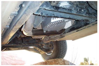
On this 1997 Hummer H1 Turbo Diesel, the PML 4L80E pan, part number 9437, holds approximately 7.5 quarts of oil compared with 5 quarts for the stock pan.
