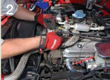
The new covers are taller to accommodate taller rockers. The raised fins also add to the height. Because the truck has A/C mounted right over the valve cover, the compressor needs to be removed so that we can trim the back of the mount. The serpentine belt's tension is released and the compressor is unbolted. Tech advisor at large Marcel Venable of Venable Concepts tackles the job with ease.
