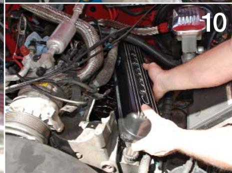
The supplied Allen bolts are secured. Because of the thicker material and internal structure of the valve covers, only two bolts are needed per cover. This allows for a cleaner look and the ability to cast scripted logos and maintain the center bolts.
