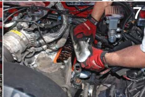
Gasket sealer is applied to the inside of the new valve covers.
