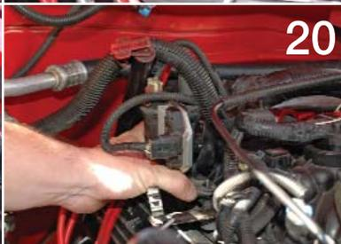
The coil is screwed onto the new raised mounts.
