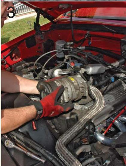
The EGR tube is disconnected from the intake manifold as is the upper radiator hose. The fairly fresh coolant is collected for reuse later. An empty beer bottle does the trick, and chances are you have plenty of them in your garage to use.
