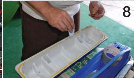
A fresh set of gaskets is stretched and fitted to the covers. Duct tape the gasket to the valve covers and set them out in the sun for a little bit to allow the sealer to dry. The last thing you want is an oil leak.
