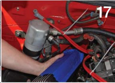
The passenger side valve cover is test fitted. We covered them with blue painter's tape before fitting to make sure no scratches occurred.
