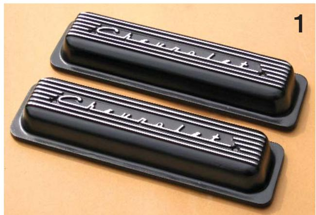
Supply. Installing aftermarket valve covers on a newer engine can be a bit of a challenge, so follow along as we bolt on some old school covers to finish off the motor of our retro-inspired C/K truck. ■
