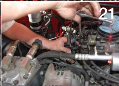
All of the wiring is plugged back in on the passenger side and the brackets are reinstalled.
