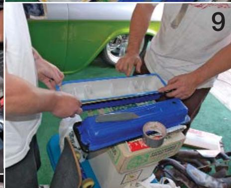
The tape is removed and the new valve cover is installed. An extra set of hands can help keep all of the accessories out of the way to avoid scratching the clean black powder coated covers.
