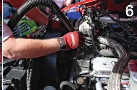
The old, scratched "polished" valve covers are removed as well as the old gaskets.
