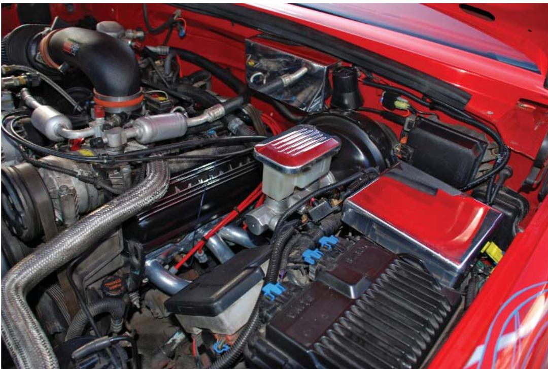
*(Below) Here are the center bolt valve covers from PML. The sand-cast aluminum covers were powder coated black with brushed raised fins and retro Chevrolet script.*
