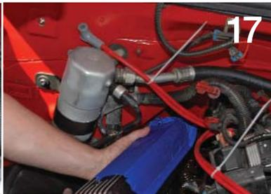
The passenger side valve cover is test fitted. We covered them with blue painter's tape before fitting to make sure no scratches occurred.
