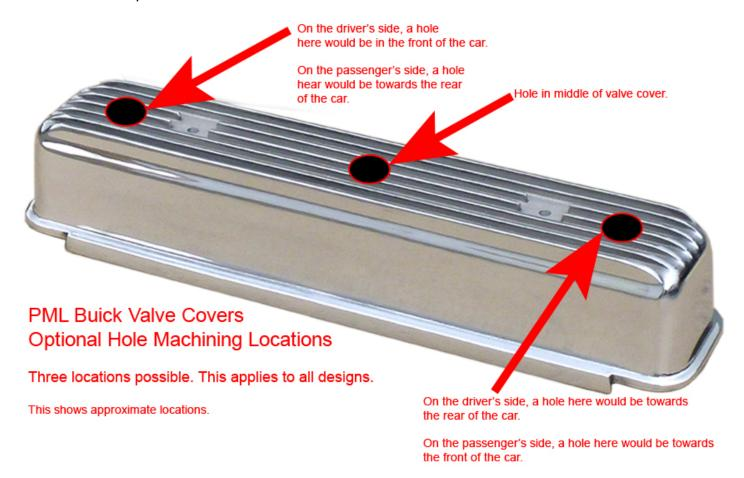
PML machines the holes to a diameter of 1½ inches. The holes are spot faced for a good seal with the grommet. For oil fill, most folks remove the PCV or breather and fill there. PML can also drill and tap for an oil cap.
