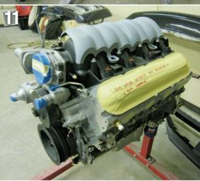
The B&M transmission and LS3 engine have been smoothed and prepped for paint. We will cover that next time, but take note of the masking on the valve cover area to ensure no areas are missed.
