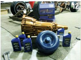
The LS3 engine is filled with Royal Purple synthetic engine break-in oil, while the transmission will get a dose of Max ATF fluid also from Royal Purple, and then the two are mated.
