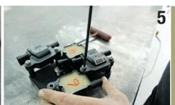
The coils are installed onto each of the mounts in an alternating pattern.
