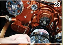
The brackets have been painted to match, and the idler pulley from Eddie Motorsports is installed with the bracket bolting to the Edelbrock water pump. This is the "No A/C" option. A Sanden compressor and bracket would be installed here if you chose that route.
