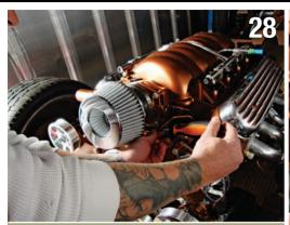
Topping things off, a Spectre Performance air filter is mounted to the painted throttle body. A custom Pro Fab air intake system will be built once the body is on the chassis.
