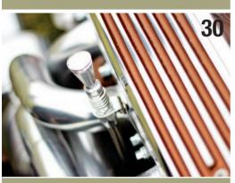
For a clean and classic oil dipstick, a Lokar Anchor-Tight locking flexible dipstick was mounted off of one of the header bolts. These dipsticks have a locking mechanism similar to an air hose disconnect that holds vacuum better and is NHRA approved. They are available in several finishes.
