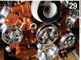
The final item, before a belt, of course, is the tensioner. The cover has been painted to fit with the theme where only the polished pulleys stand out.
