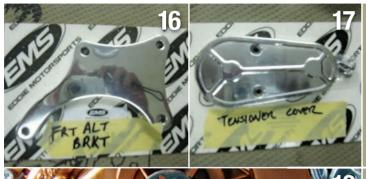
The next step is the front drive accessory setup. Eddie Motorsports makes its SDrive setup featuring all of the brackets, pulleys and accessories needed for a variety of applications. We opted for its polished kit to offset the BASF Infiniti Copper Metallic flat paint on the engine.
