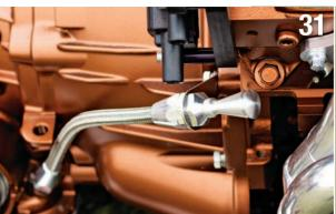
A Lokar transmission dipstick is also used. It mounts off of the housing out of the way.
