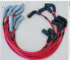
Mast Motorsports supplies a set of spark plug wires that is the correct length for the newly relocated coils.
