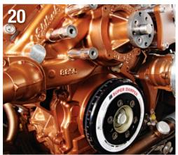
The Edelbrock high-performance water pump has been smoothed and painted to match, except for the contact areas, and installed. The pump maximizes and equalizes flow for high-performance cooling.
