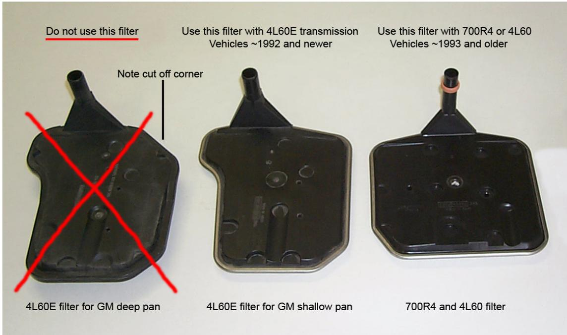
This pan is designed to work with the 4L60E and 700R4 filters that fit the GM shallow pans. These filters are seen above in the middle and on the right.
