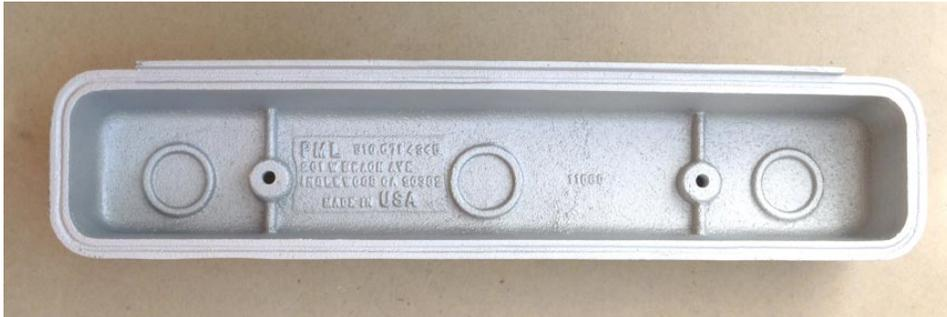
Image of the interior of these valve covers showing the reinforced rings for machining:
